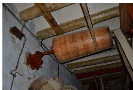
Wheels that transmit the energy of water to the machines.
