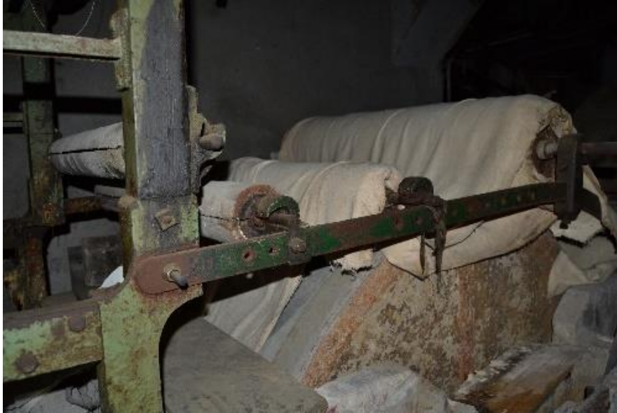
Side view of the first paper machine with the main drum and four axes of transmission of the wet leaf
